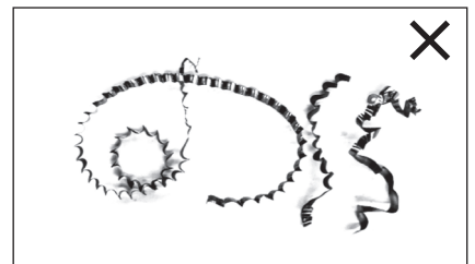
Continuously coiled long chips
